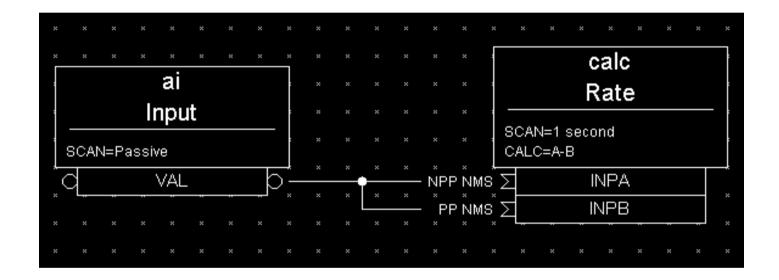
INPA fetches data that is 1 second old because it does not request processing of the AI record. INPB fetches current data because it requests the AI record to process. The subtraction of these two values reflects the 'rate of change' (difference/sec) of the pressure reading.
