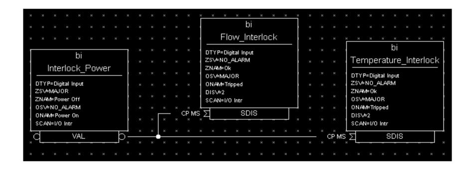
If chassis is powered off, Temp Trip and Flow Trip indicate Normal. Force these PVs into an alarm state by specifying .SDIS with .MS (maximize severity) to the Chassis On record. Set .DISV (disable value) to 2 so processing will never be disabled.
