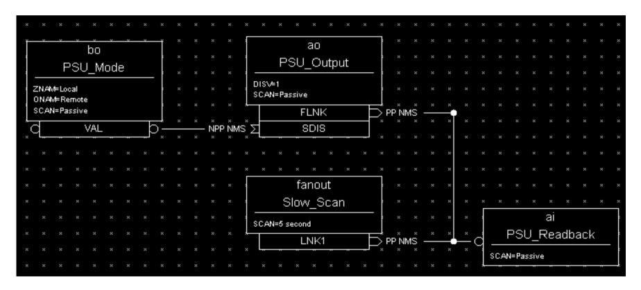
The AI record gets processed every 5 seconds AND whenever the AO record is changed. This provides immediate response to an operator's changes even though the normal scan rate is very slow. Changes to the power supply settings are inhibited by the BO record, which represents a Local/Remote switch.
