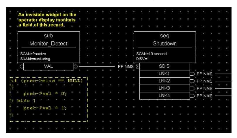
If no CA monitor exists on the SUB record (i.e. the operator logs out), MLIS will be NULL. The subroutine will then set the .VAL field to 0, causing the sequence record to process.
