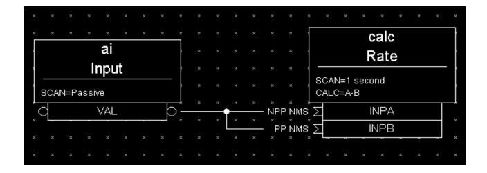
INPA fetches data that is 1 second old because it does not request processing of the AI record. INPB fetches current data because it requests the AI record to process. The subtraction of these two values reflects the 'rate of change' (difference/sec) of the pressure reading.
