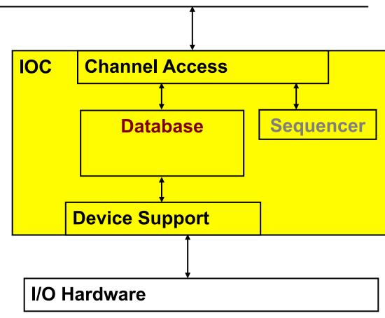
"Hard" IOCs run vxWorks and directly interface to A/D, D/A, LLRF, ... hardware.
