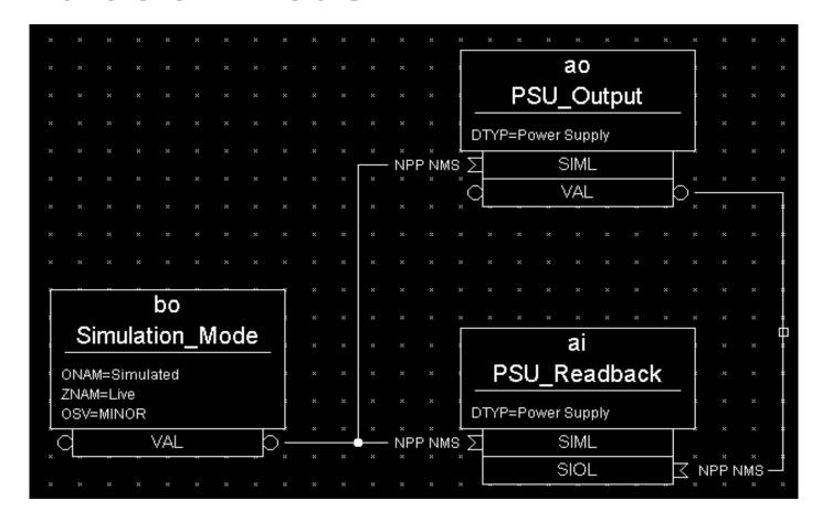
When in simulation mode, the AO record does not call device support and the AI record fetches its input from the AO record.
